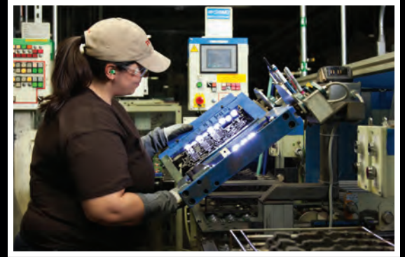
Production Team Member Jessica Weaver performs the final visual check for transmission valve bodies before they are sent for assembly.
